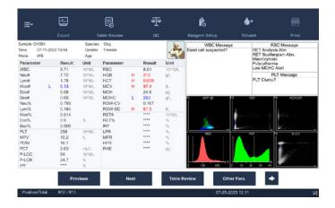
**NOTE:** During the analysis process, if errors like a clog or bubble occur, the analyzer will automatically display the results of related parameters as invalid, and alarm information will show on the error information area. See *Section 11: Troubleshooting the Analyzer* for the way to remove errors.
