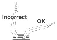
**NOTE:** Position the sample barcode reader properly facing the barcode label. Otherwise, a wrong reading may occur.
