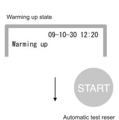
The LCD indicates [Tests reserved], and the analyzer is set to start automatically when the analyzer is ready.
