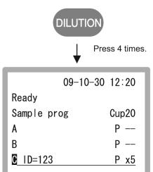
c. Press **SAVE** to accept the sample programming for Sample C.
