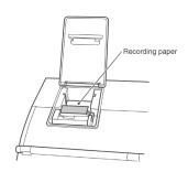
**NOTE:** Pass the paper through the opening of the printer cover and close the cover.
