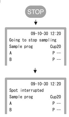
2. By pressing **STOP** during interrupted stage, all remaining test programming will be canceled. The LCD turns to [Ready]. All the Sample indicators are turned off.
