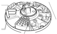
Sampler leak check tip
