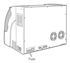
2. Pull out the fuse holder by turning it 1/4 turn counterclockwise using a screw driver. If the fuse has burned out, replace it with a new one. Insert the fuse holder and lock it by turning it 1/4 turn clockwise.
