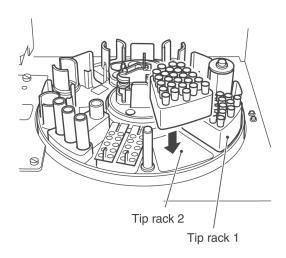
7. Press **TIP/CUP** to complete the replacement mode. The sample carousel turns the sample racks.
