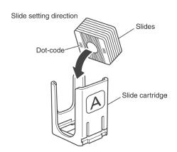
3. Place slides to be tested, dot-code surface down, in the slide cartridge. Be sure to put the slide weight on top of the stacked slides.
